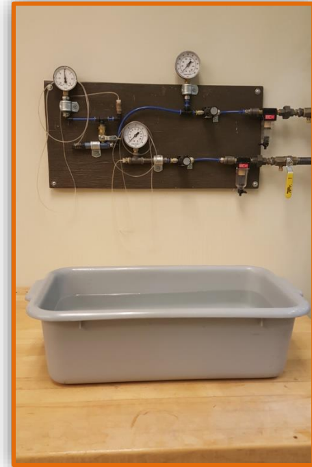
Pressure/Vacuum leak station
